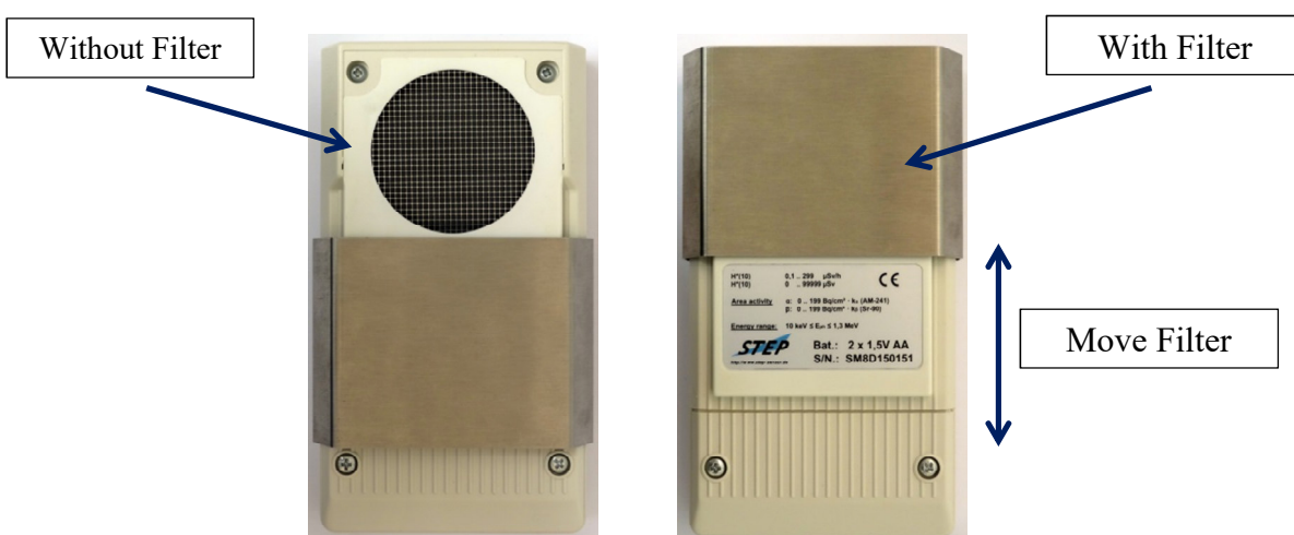
Fig. 4 Backside of Survey Meter SM 8 D without (left) and with (right) energy compensation filter
