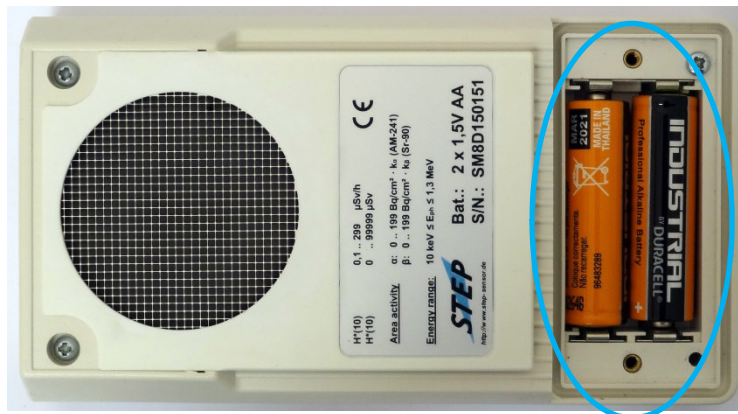
Fig. 3 Battery Survey Meter SM8D with batteries
