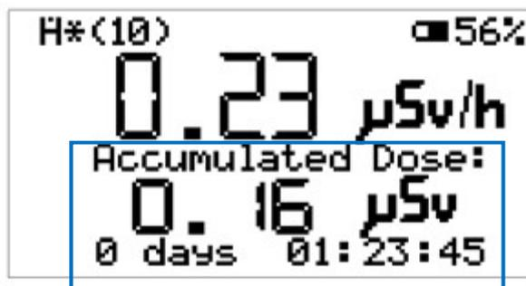
**Fig. 7)** Mode “dose rate“: Display “Accumulated Dose”.
