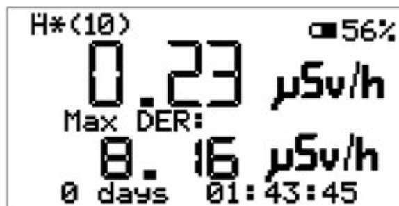
Fig. 16) Display in the measurement mode  $\mu\text{Sv/h}$ .
