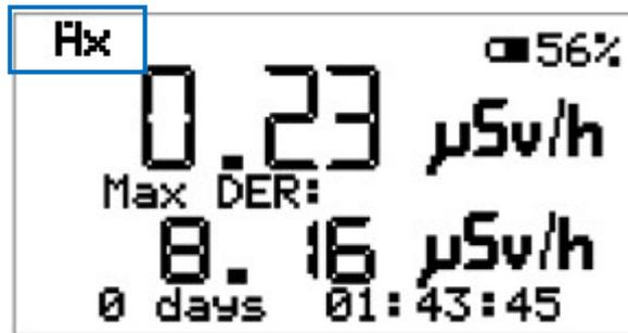
The factor of the applied ionisation chamber of OD-02 / OD-02 Hx amounts to approx.  $4.2 \text{ fA}/\mu\text{Sv}\cdot\text{h}^{-1}$ . The current generated by the ionisation chamber is transformed into processable voltage by means of the probe electronics. For that purpose, a transimpedance amplifier converts the current via a switchable feedback network into a proportional voltage signal. This voltage signal is scanned in steps of 80 ms in both dose rate modes.
