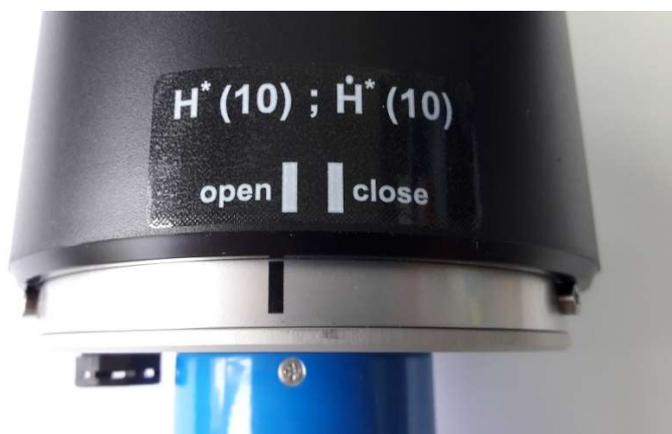
**Fig. 14)** Interlock of the wall reinforcement cap
