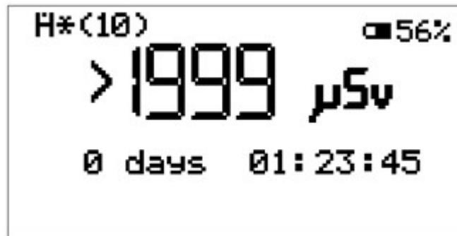
Fig. 18 b) Display overflow of measurement range in mode „Dose“.
