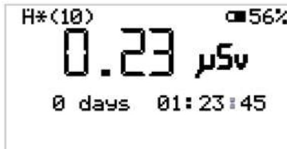
*Fig. 17) Display in the dose measuring mode µSv.*
