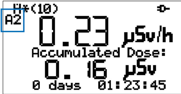
*Fig. 29) Alarm threshold A2 is reached at the moment (symbol "A2" flashes)*
