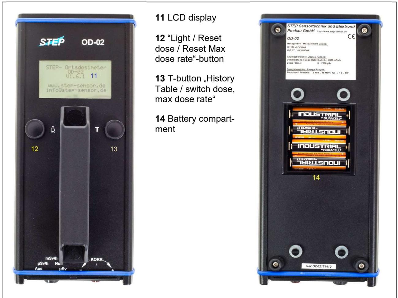
Fig. 3) Control elements front and rear side
