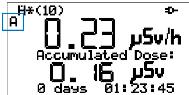
Fig. 28) Alarm threshold(s) activated
